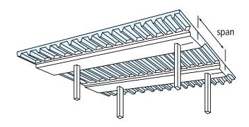
As with solid slab arrangements, the band beam has a relatively wide, shallow cross section which reduces the overall depth of floor while permitting longer spans.
